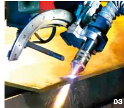
Plasma bevel cutting with the VBA EXPERT PRO.
