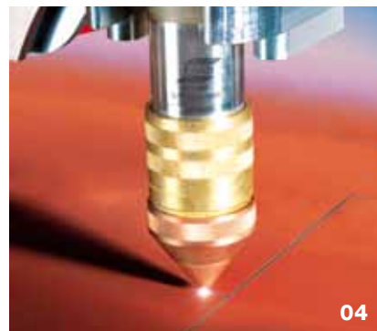
Plasma cutting and marking with the same torch.
