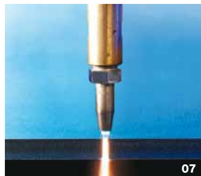
Oxy-fuel cutting up to 8 inch thick material.
