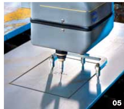
Pin marker for lettering and numbering. Ideally suited to mark before / after painting, before part treatment.
