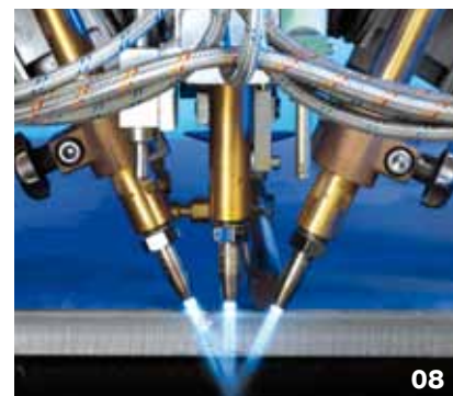
Programmable angle oxy-fuel bevel cutting with infinite rotation.
